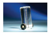
Perspex syringe shields for the shielding of beta radiation. The syringe is polished on the inside to guarantee a clear view on the syringe. The syringe is fixed with 2 Teflon screws. The syringe shields will be made to fit the syringe models you are using.
